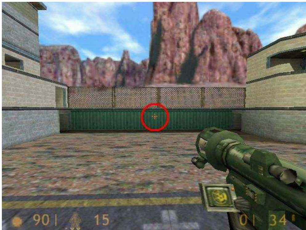
Figure 6.13: Monitoring the effect of network latency in Half-Life — the weapon's laser sight (the circled red dot) is calculated server-side
